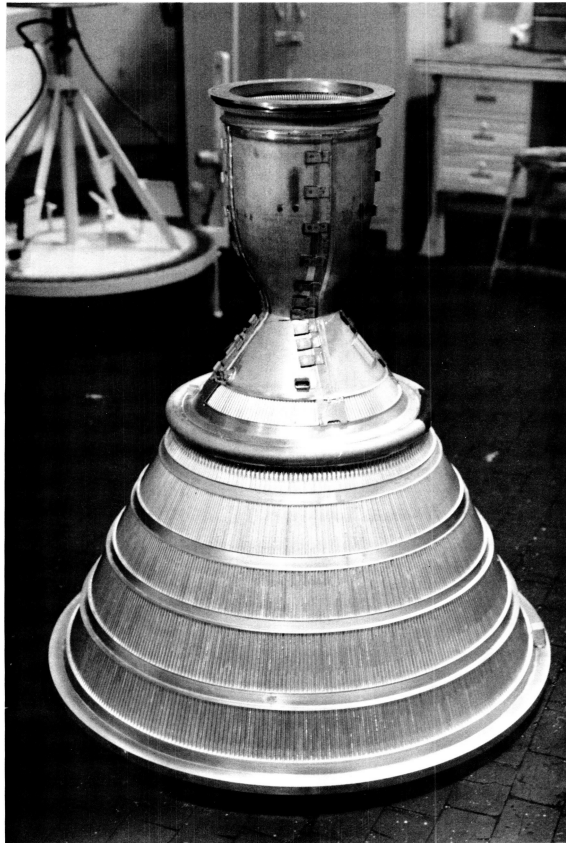
Figure 60. Brazed Assembly After Removal From Mandrel
