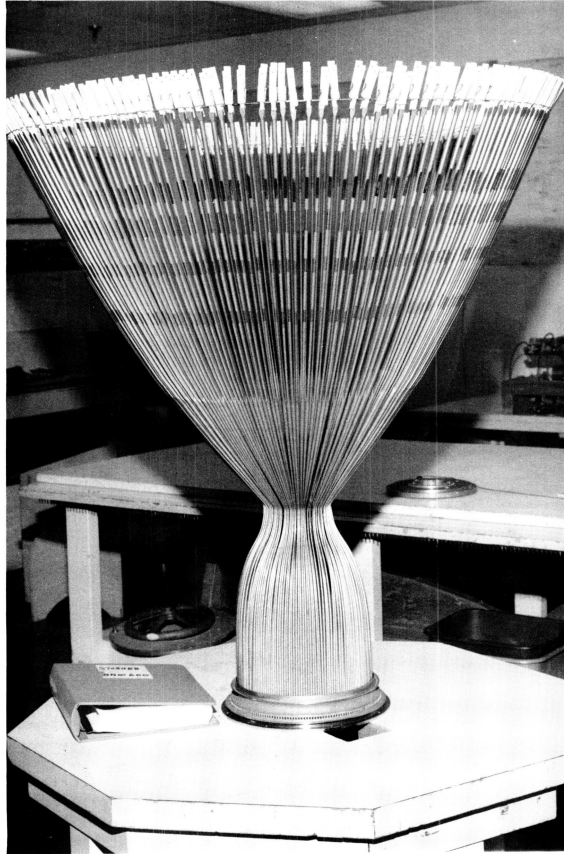
Figure 44. Long Tubes Stacked in Exit Manifold
