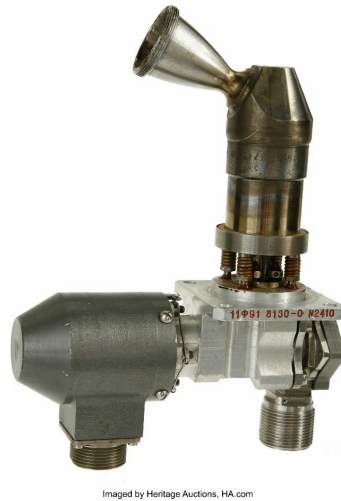
Figure 2.4: The Soyuz capsule's hydrogen peroxide yaw thruster.
